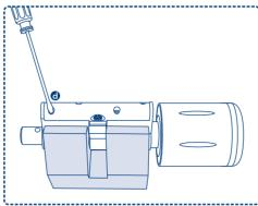
① Slide cylinder into assembly holder. ②Loosen all screws ② on bridge with flathead screwdriver.
