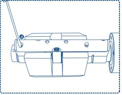
8 Tighten bridge screws with flathead screwdriver.
