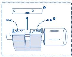
2 Remove bridge from the top of cylinder carefully. There are two steel balls in between. Please keep steel balls in a container to prevent from loss during the length adjustment.
