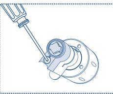
5 Tighten screw of connect body set on Reader Knob part and Inner Knob part with Phillips screwdriver.
