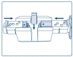
**6** Assemble three parts: Reader Knob part, Cam, and Inner Knob part.
